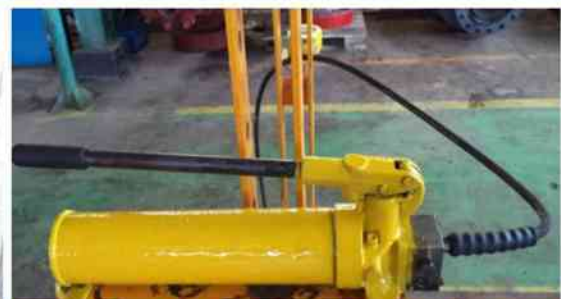
ENERPAC / HYDRAULIC TOOLS Cap. 10 TONS
