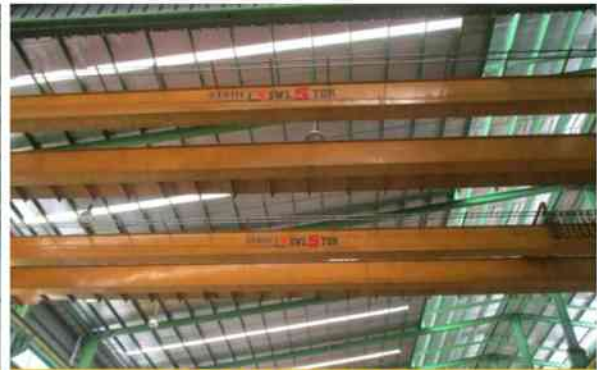
OVERHEAD CRANE CAP. 5 TON
